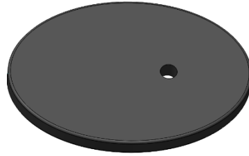
Figure 4.2: Oval valve membrane with offset through hole.
