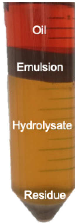
Figure 2.1: Centrifugally fractionated slurry of the bioprocessed salmon by-products
