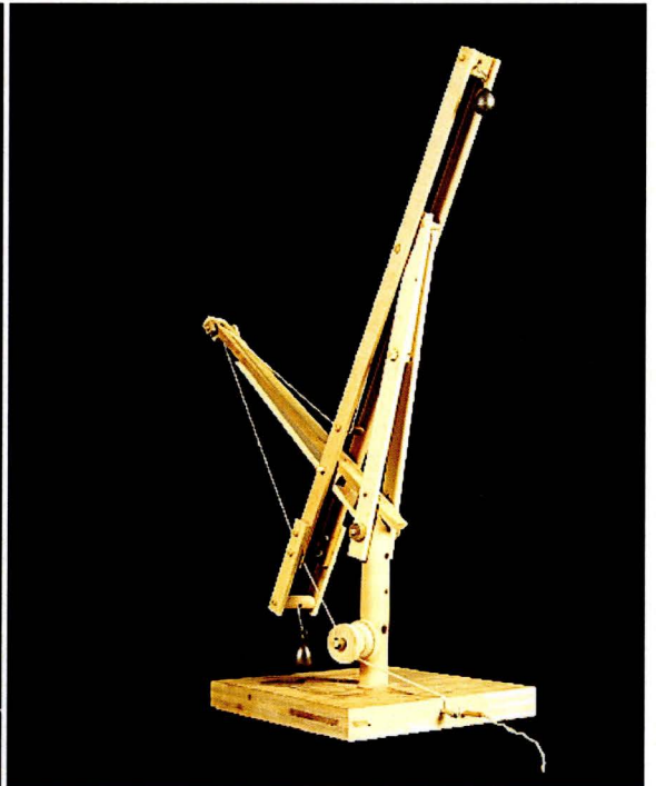
Frame featuring two bent-wood trusses pre-tensioned to pull away from one another, resisted by a tensile link.
