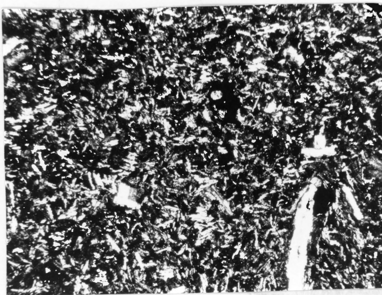
Plate X. Sample no. A; (x 2.5, crossed polars). Spilite. Feldspar phenocrysts within pilotaxitic groundmass.
