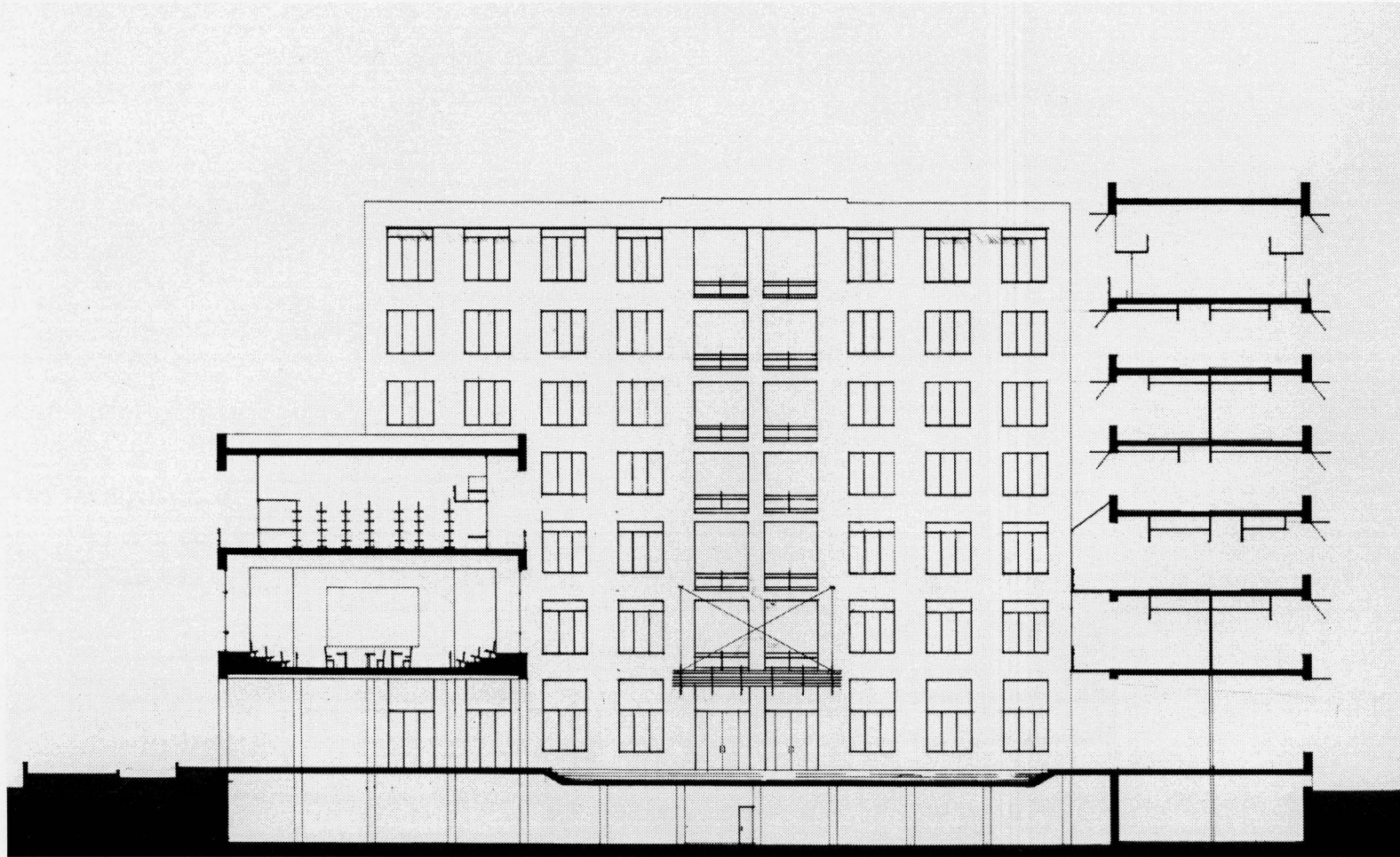
Figure 32: Section through the House of Chiefs chamber and library and also through the parliamentary block on the other side of the kgotla space. Both libraries pull away from the edge of their respective buildings, enabling the establishment of balconies that look out to the outside, and are used as study areas. The administration office elevation opens up in the centre into the kgotla . In the basement is parking and a kitchen that serves the restaurants in the complex.
