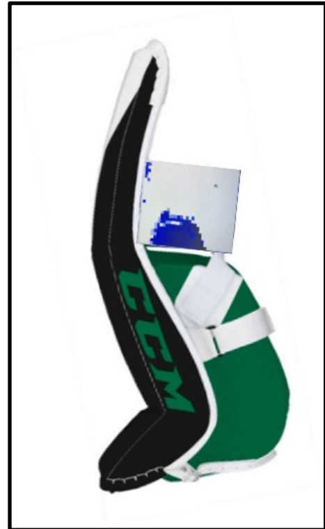
Figure 16. Simulated overlay of Tekscan pressure sensor output on medial knee stack.
