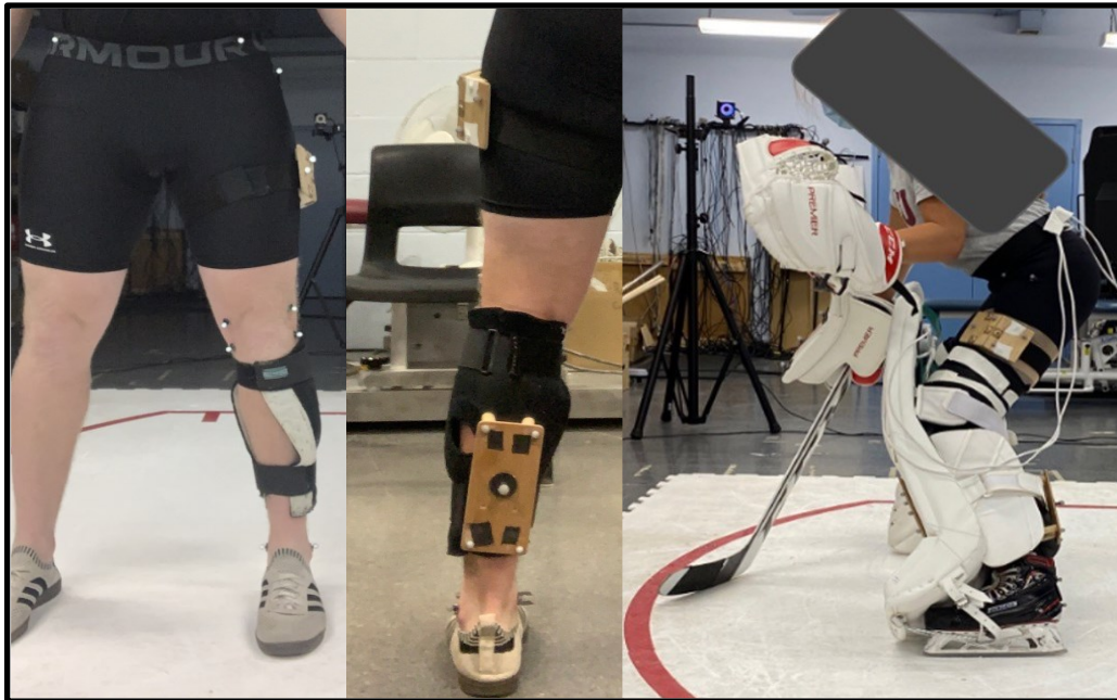
Figure 19. Left: Anterior view of calibration trial marker setup. Middle: Posterior calf rigid body. Right: During the pad condition trial the calf rigid and upper thigh rigid bodies as well as skate and hip individual markers remain on the participant.
