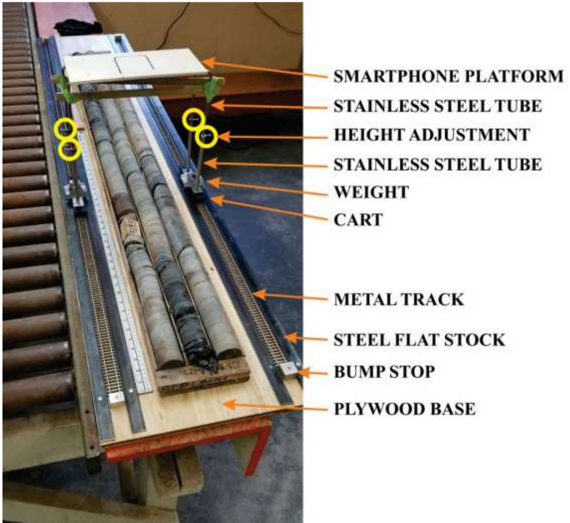
Figure F1: Core photography gantry apparatus.
