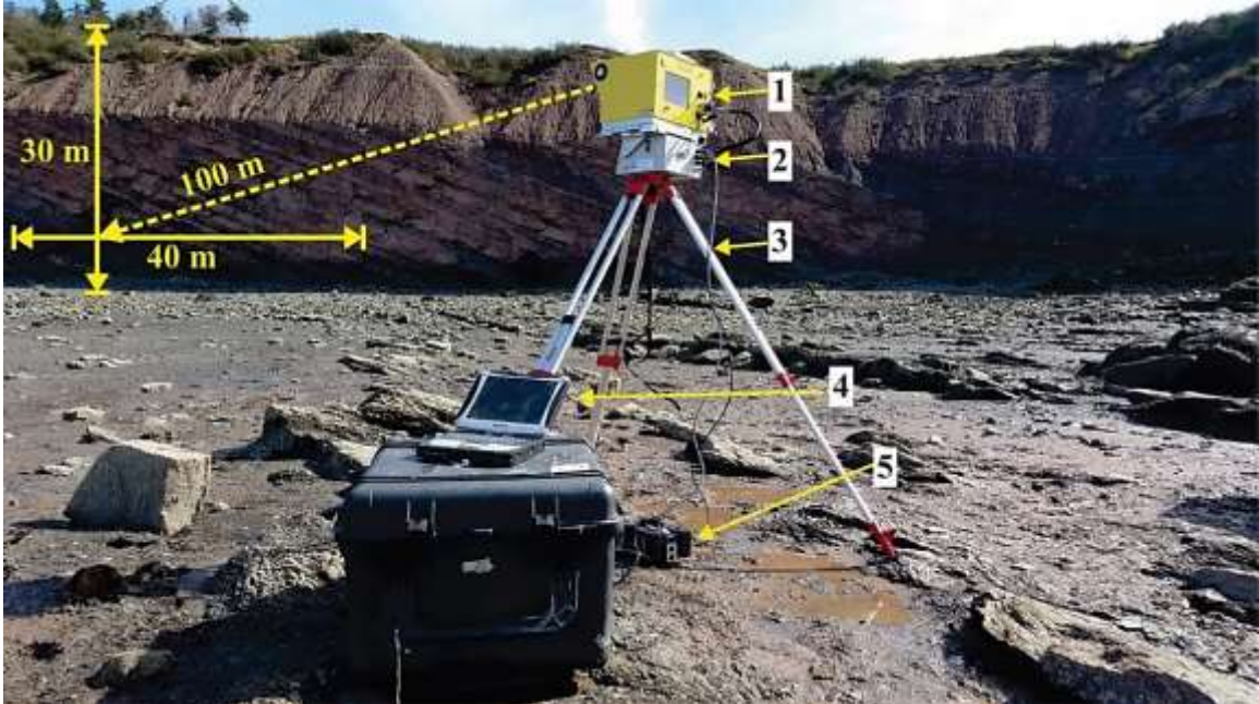
Figure 2.4: A photograph of the Optech ILRIS-3D lidar scanner setup at Joggins, Nova Scotia (Kelly and Wach 2020). Labelled in this photograph is the laser scanner (1), which was mounted atop the pan/tilt base (2), both of which were connected to a tripod (3). A ruggedized laptop computer (4) was used to adjust scanner settings and initiate the lidar scan. The lidar unit (1 and 2) is powered by a battery pack (5). The dipping strata of the Joggins Formation can be seen in the background. The distance from the lidar setup to the outcrop was approximately 100 m and is indicated by the dashed line.
