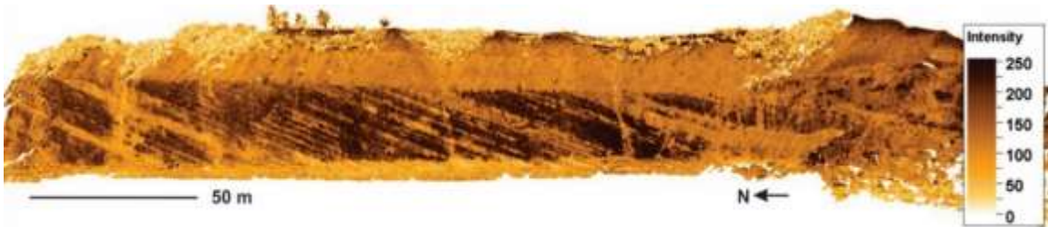
Figure 3.16: The generated point cloud cliff section viewed from the West. A colour scale has been applied based on the intensity of the reflected light, which ranges between 0 and 255. The lower intensity values correlate with the finer-grained, quartz-poor lithologies and unconsolidated sediments. The higher intensity values correlate with the good quality quartz sandstone, as well as vegetation and sandstone-rich mine tailings.
