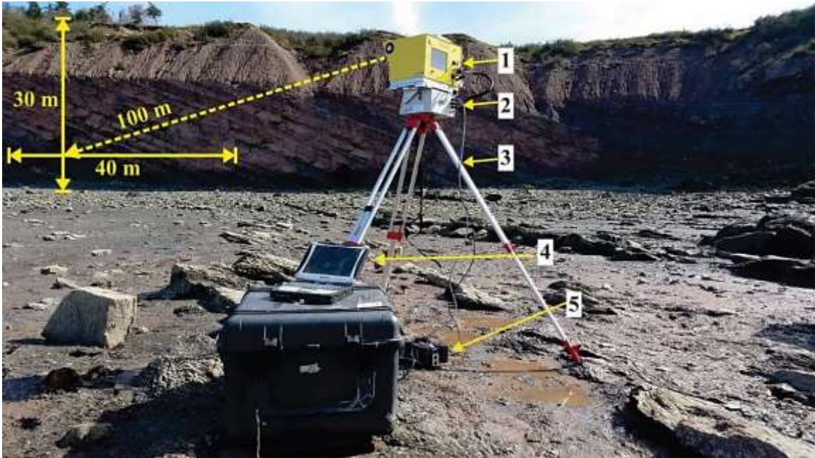
Figure 3.6: An image of the Optech ILRIS-3D lidar scanner setup. In this image, the laser scanner (1) is mounted atop the pan/tilt base (2), both of which are connected to a tripod (3). A ruggedized laptop (4) is used to adjust scanner settings and initiate a scan. The lidar unit (1 and 2) are powered by a battery pack (5). The tilted strata of the Joggins Formation can be seen in the background. The distance from the lidar setup to the face of the outcrop is approximately 100 m and indicated by the dashed yellow line.
