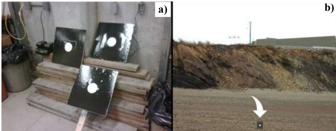
Figure 2.6: Images of the utilized georeferencing targets. (a) image of the lidar georeferencing targets that are placed at varying X, Y, and Z coordinates in front of the cliff face portion to be scanned (Rafuse and Wach 2011). (b) image showing the placement of one of the georeferencing targets on the inter-tidal zone with the cliff and the Joggins Fossil Centre in the background (Rafuse and Wach 2011).
