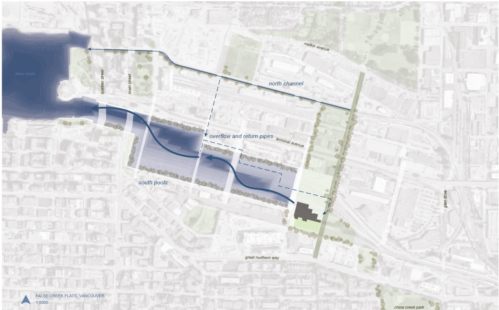
Site plan of the Flats showing outer edge of water in the pools. This water level occurs during storm events that bring large quantities of precipitation as well as potential tide rises. The outer edge protects up to 5 meters in elevation.
