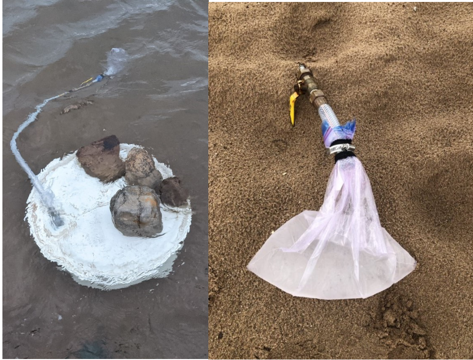
A 1 Field photographs of installed seepage meter (left) and seepage meter bag full of water from SGD.
