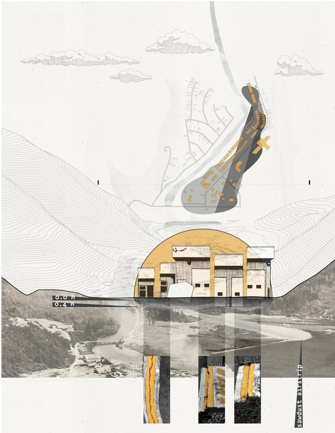
Hybrid drawing showing the areas within Tahsis suffering from the former sawdust dumping site and buildings in danger of seismic issues due to significant ground settling.
