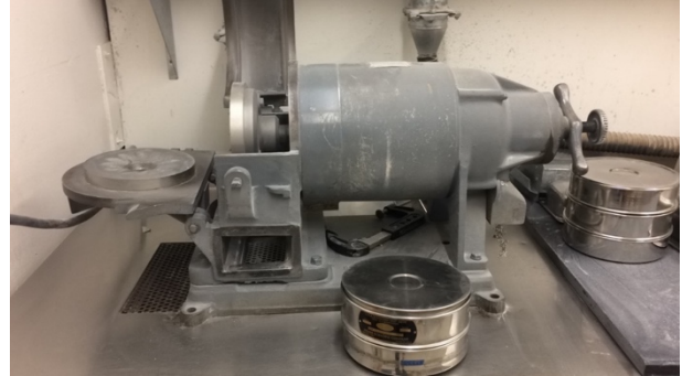
Figure 15; Disk mill used in the initial stage of crystal isolation. Sieve used was for 250 micrometers.
