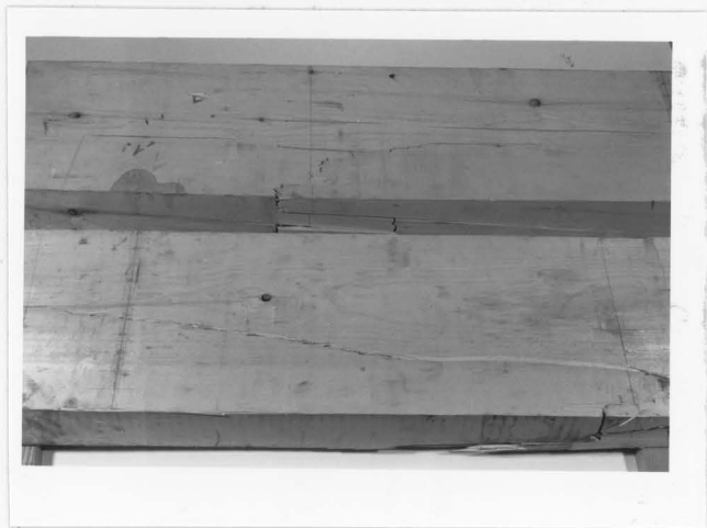
FIG. B.55 TYPICAL FAILURE IN 4 x 12 CLEAR BEAMS SUBJECTED TO THIRD-POINT LOADING
