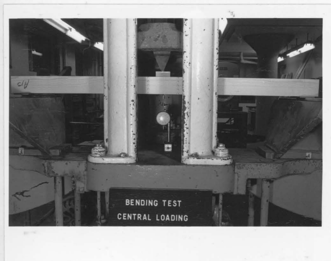
FIG. 4.7 SET-UP FOR BENDING TEST WITH CENTRAL LOADING
