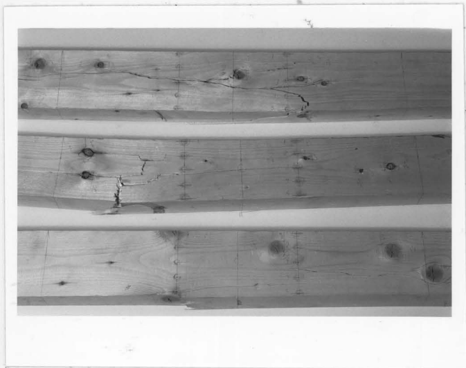
FIG. 4.10 TYPICAL FAILURE IN 2 x 4 KNOTTED BEAMS SUBJECTED TO THIRD-POINT LOADING
