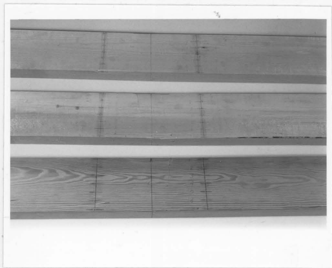
FIG. 4.9 TYPICAL FAILURE IN 2 x 6 CLEAR BEAMS SUBJECTED TO CENTRAL LOADING
