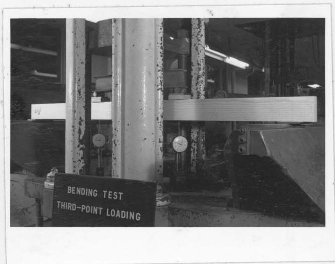
FIG. 4.6 SET-UP FOR BENDING TEST WITH THIRD-POINT LOADING
