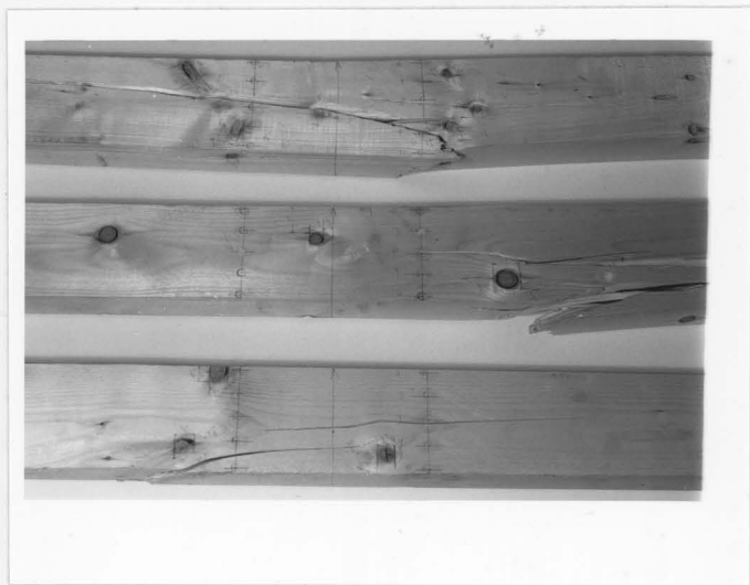
FIG. 4.11 TYPICAL FAILURE IN 2 x 4 KNOTTED BEAMS SUBJECTED TO CENTRAL LOADING
