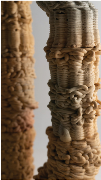
Figure 45: Close up of interrupted vessels stacked. Surface articulated through air modulation and physical interruptions.
