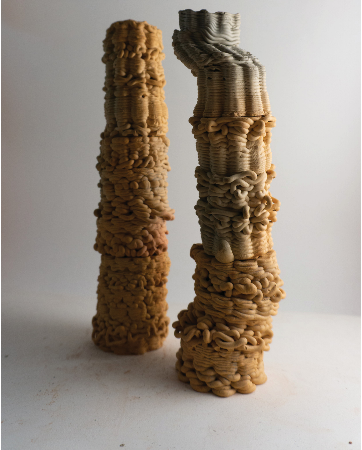
Figure 46: View of interrupted vessels stacked. Surface articulated through air modulation and physical interruptions.
