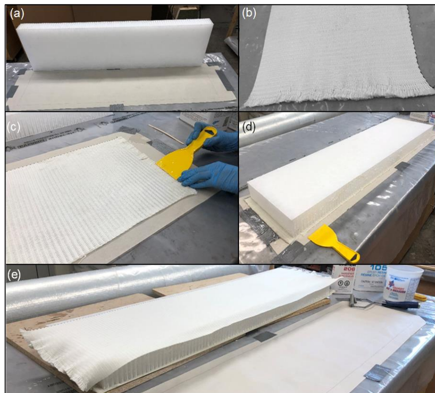
Figure 1: Fabrication of sandwich panel: (a) parchment paper taped on table surface; (b) fabric cut to the required length; (c) layer of fabric placed on epoxy layer; (d) core component placed on second layer of spread-evenly epoxy; (e) second FRP facing component set on PP core.
