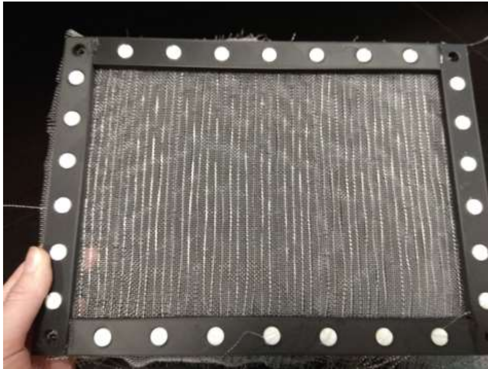
Figure 4.1 Nylon plastic mesh collecting electrode (C8) with 12.5% of stainless steel wires
