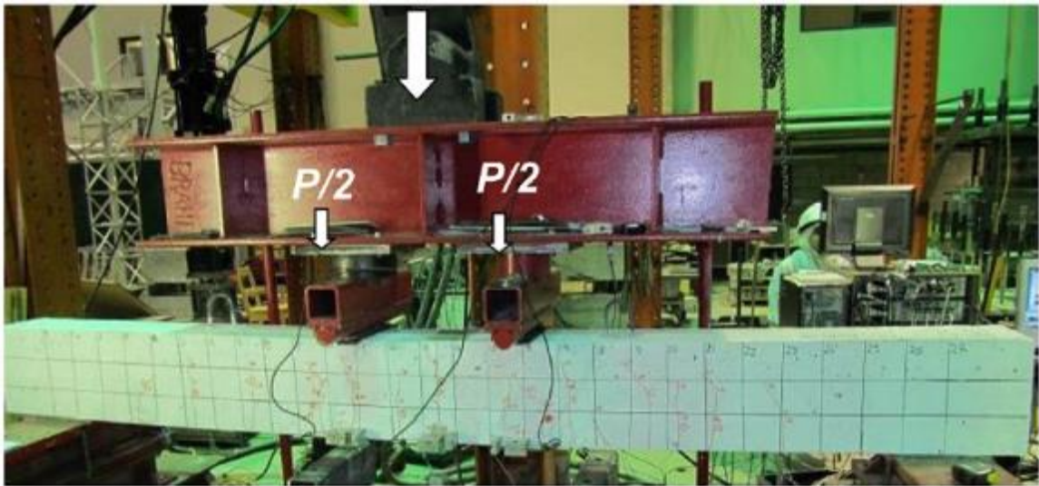
Fig 2-7 Beam during four-point bending test (Elgabbas et al. 2016)
