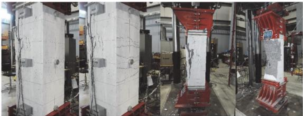
Fig 2-13 Failure pattern of GFRP column with low eccentricity (Guerin et al. 2018)
