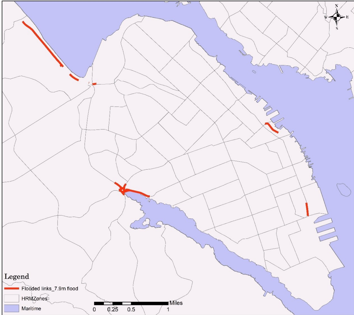
Figure A – 6 The flooded links of the Halifax Peninsula transport network under a 7.9 m flooding scenario
