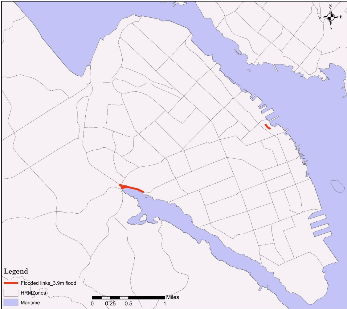
Figure A – 5 The flooded links of the Halifax Peninsula transport network under a 3.9 m flooding scenario
