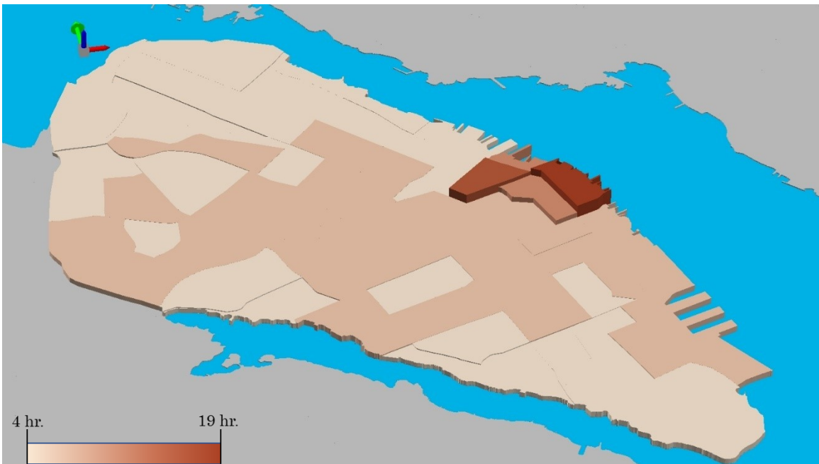
Figure B – 8 A 3-D visualization of clearance time across Halifax Peninsula TAZs when 15% auto-based demand are served by transit and school buses
