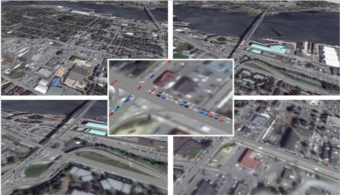
Figure C – 10 Traffic evacuation and congestion visualization within a traffic evacuation microsimulation model
