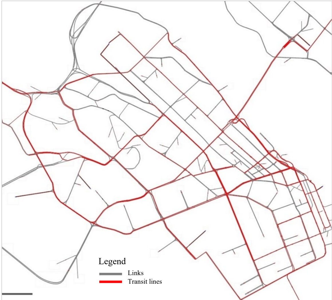
Figure 9-3 Bus routes obtained from the MILP optimization model in Chapter 5
