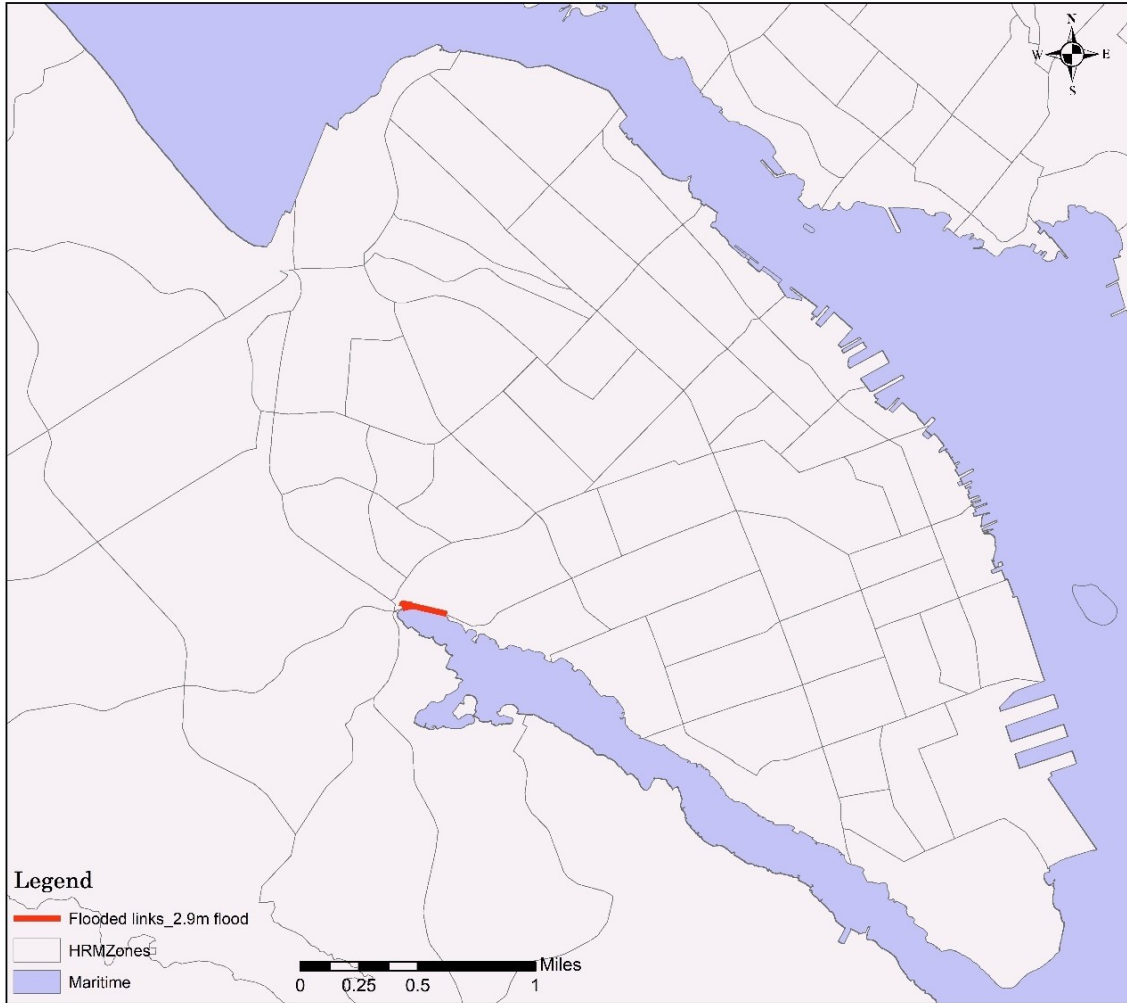
Figure A – 4 The flooded links of the Halifax Peninsula transport network under a 2.9 m flooding scenario
