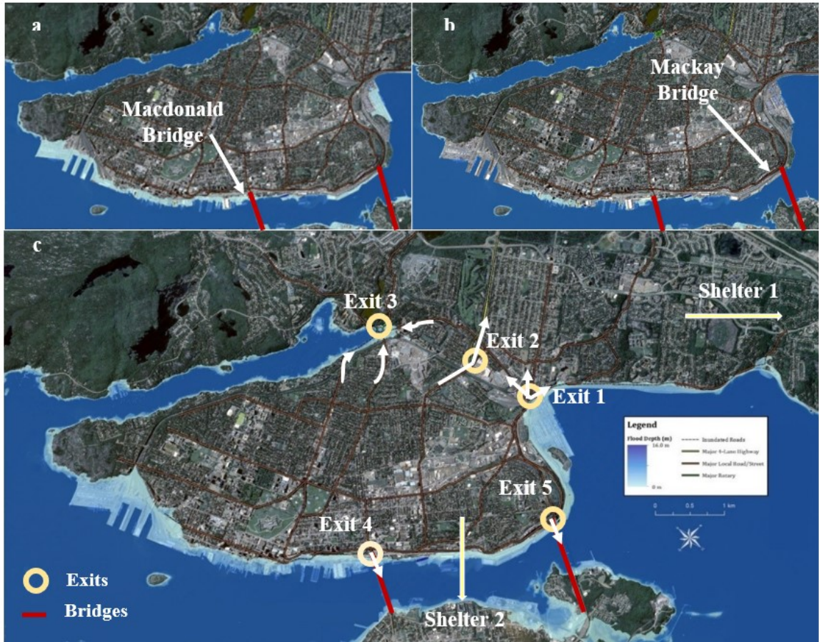
Figure 4-2 Flooding extent in the Halifax Peninsula under (a) 2.9 m, (b) 3.9m, and (c) 7.9m flooding scenarios
