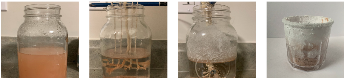
The process of separating salt from clay bodies using warm water to get white salt.
