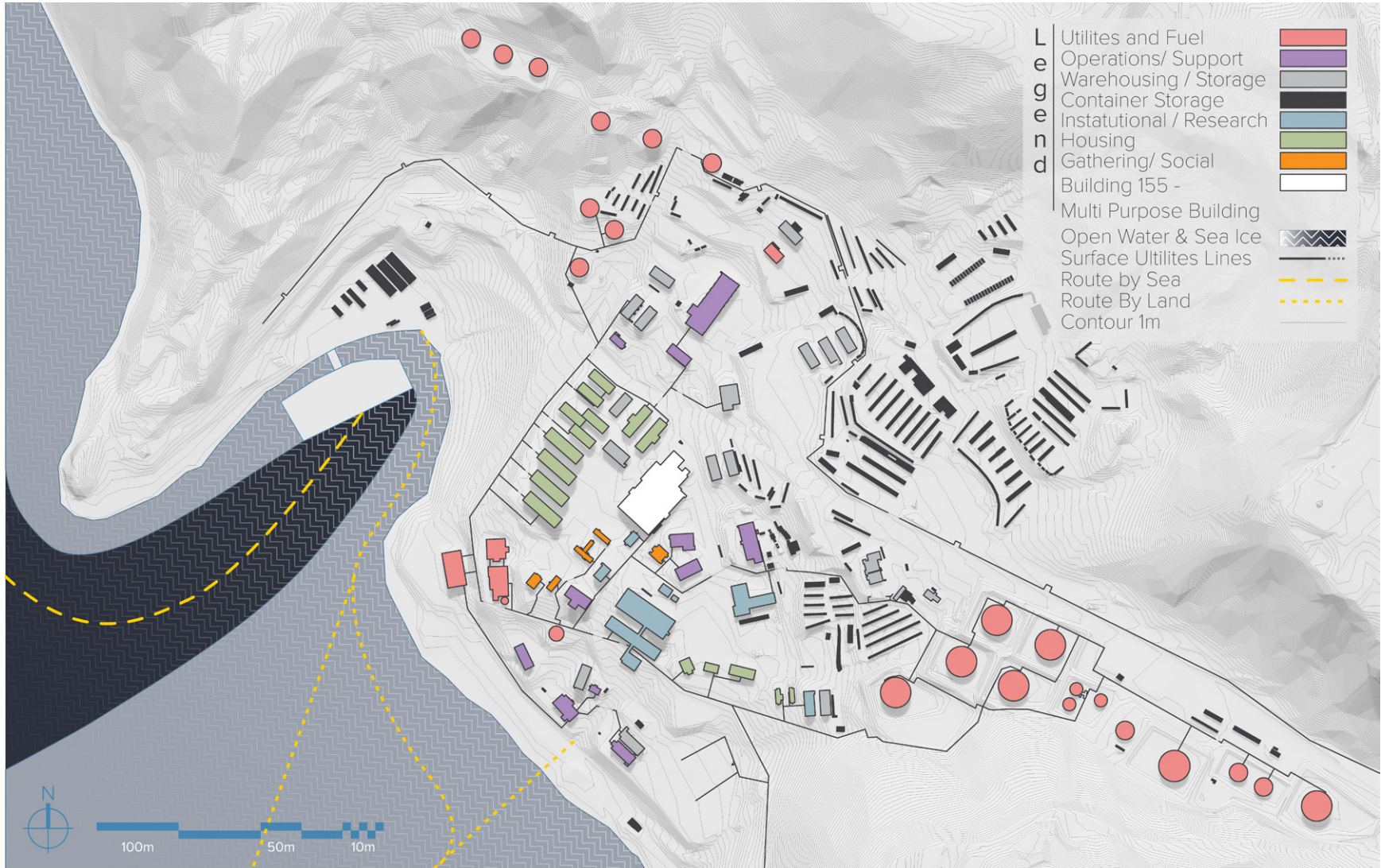
Figure 23: McMurdo Station site plan with breakdown of major programmatic spaces, map data from Lidar imaging of the McMurdo Valley, Antarctica (Fountain et al. 2017).
