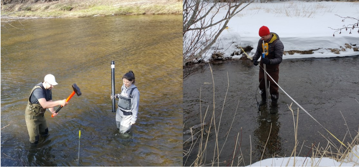
Figure 7: Installation of a stilling well in the Mabou River during May 2019 (left image). Stream gauging of the NE Mabou River in March 2020 (right image) using a Flowtracker2 Handheld-ADV (SonTek).
