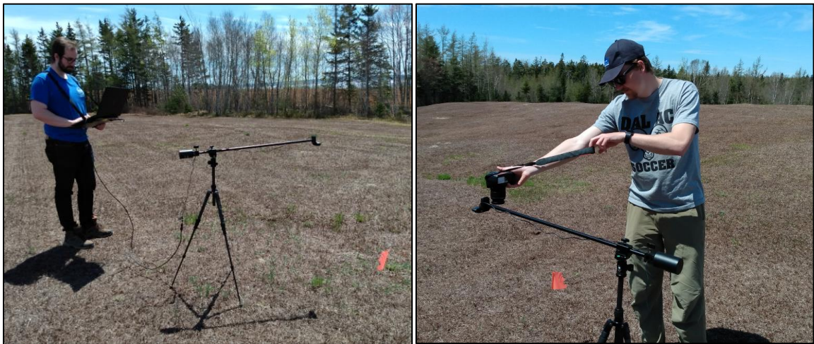
Figure 12: Field experimental setup showing image capture in the Portapique field on May 25, 2020. A tripod with an extension arm was used to hold the Logitech c920 camera at a position of 0.98 m between the lens and the ground while the laptop captured the image (L). The Canon T6 camera was held with the lens directly beside the Logitech c920 at the same height for image capture (R).
