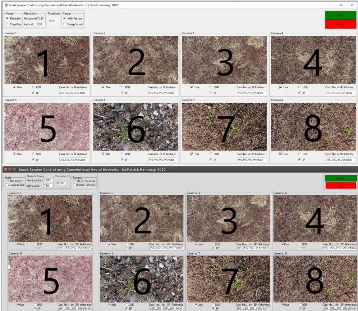
Figure 21: GUI written in Python 3.8.2 using the Tkinter library for controlling herbicide application on an 8-camera, 8-nozzle sprayer using CNNs. The top window shows the appearance on Windows 10 and the bottom window shows the appearance on Ubuntu 16.04.
