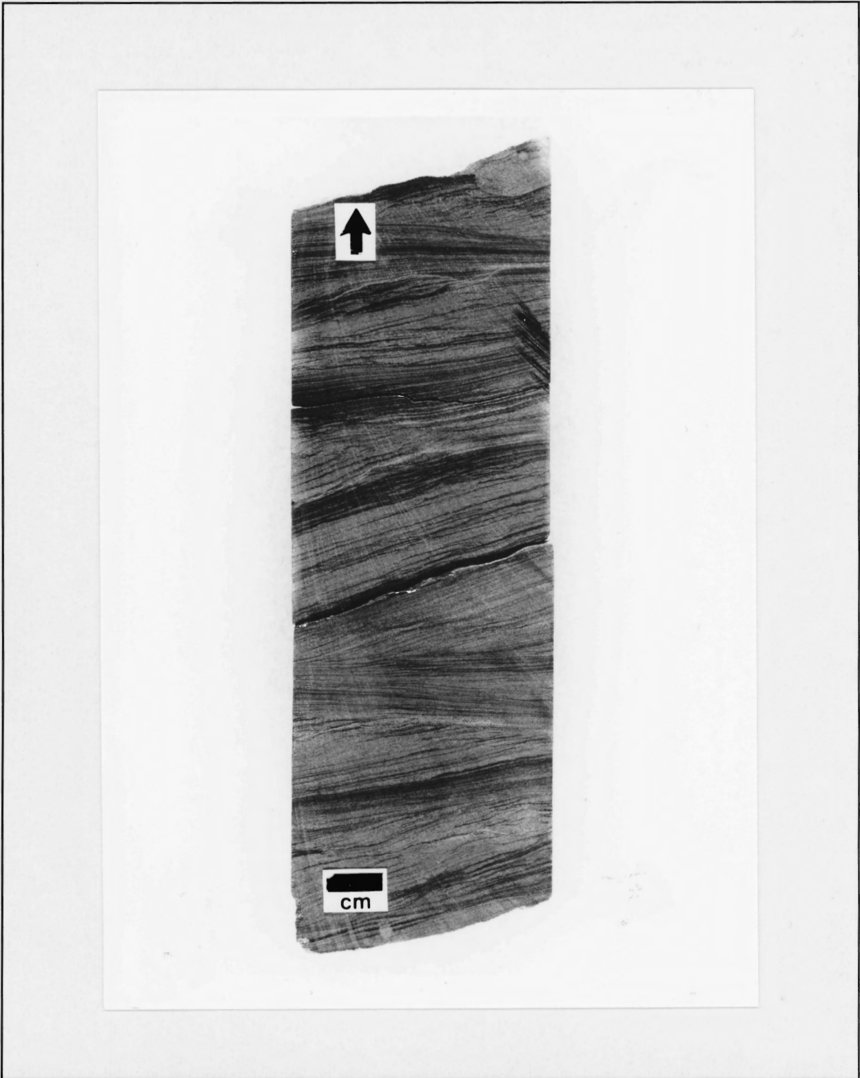
Figure 2.4 Cross-laminated sandstone facies (Sr). Note the clay partings, small cross-laminae 1-2 cm thick, and climbing ripple forms.
