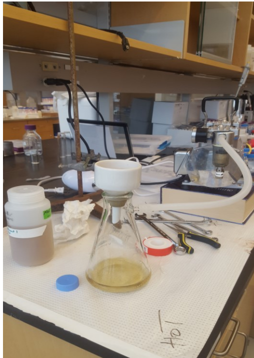
Appendix A: Filtration System for the pretreatment of raw wastewater.
