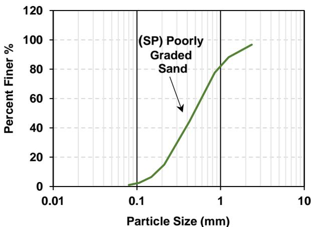
Figure 1. Gradation curve of poorly graded sand
