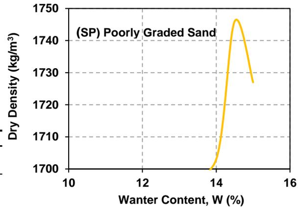
Figure 2. Maximum dry density and optimum water content
