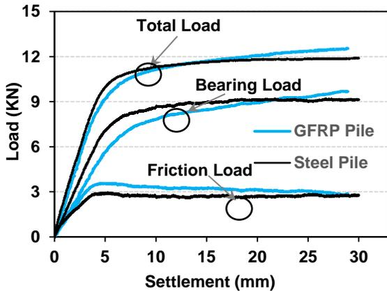
Figure 7. Pile load test results for GFRP and steel pile
