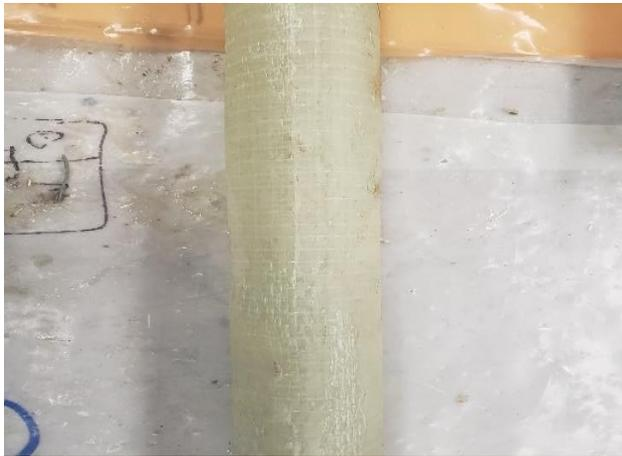
Figure 4. GFRP pile
