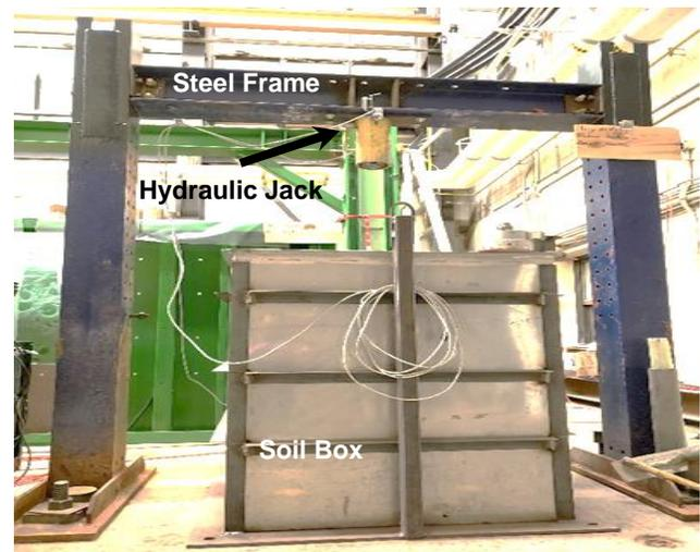
Figure 6. Pile load test set up
