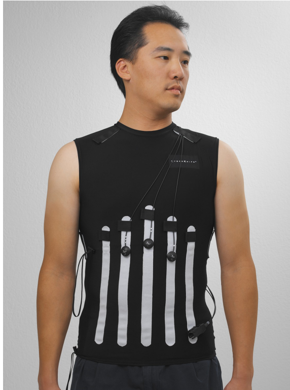
Figure 1.8: Vest used to track patient respiratory motion [30].
