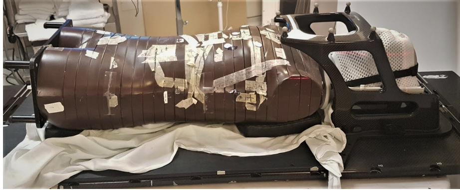
Figure 2.24: Image of the phantom set-up which used for the end-to-end test for collision detection accuracy.
