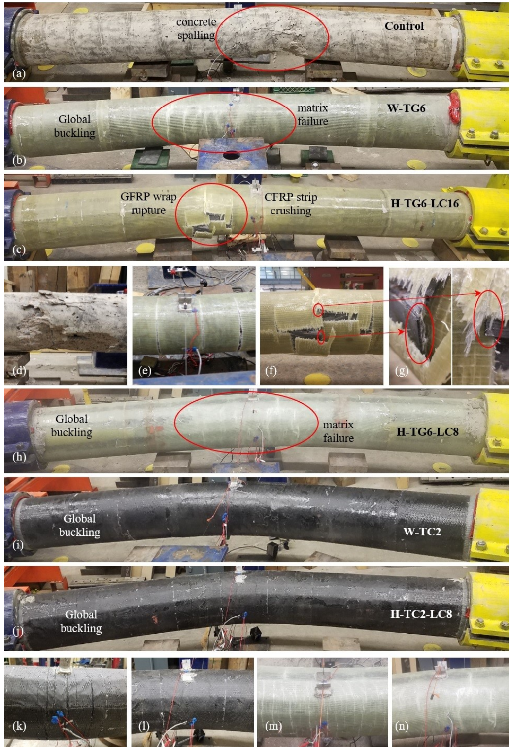
Figure 11. 4 Failure at ultimate state: (a) Control, (b) W-TG6, (c) H-TG6-LC16, (d) concrete spalling control specimen, (e) matrix rupture in W-TG6, (f) rupture of GFRP wrap in H-TG6-LC16, and (g) crushing of CFRP strip, (h) H-TG6-LC8, (i) W-TC2, (j) H-TC2-LC8, (k) matrix rupture in tensile side of H-TC2-LC8, (l) compressive side of H-TC2-LC8, (m) tensile side of H-TG6-LC8, and (n) compressive side of H-TG6-LC8
