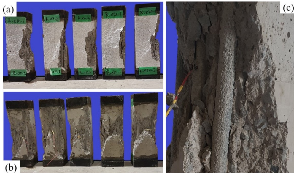
Figure 3. 4 Mode of failures: (a) side view, (b) compression side, and (c) crushed concrete and visually intact compressive rebar
