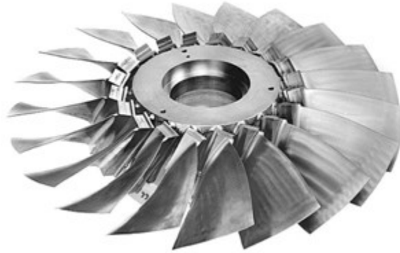
Figure 1-2 - A blisk (compressor blades and disk) created using linear friction welding [5].
