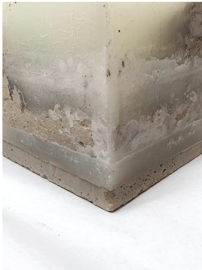
Investigation 3 - layers of wax and concrete
