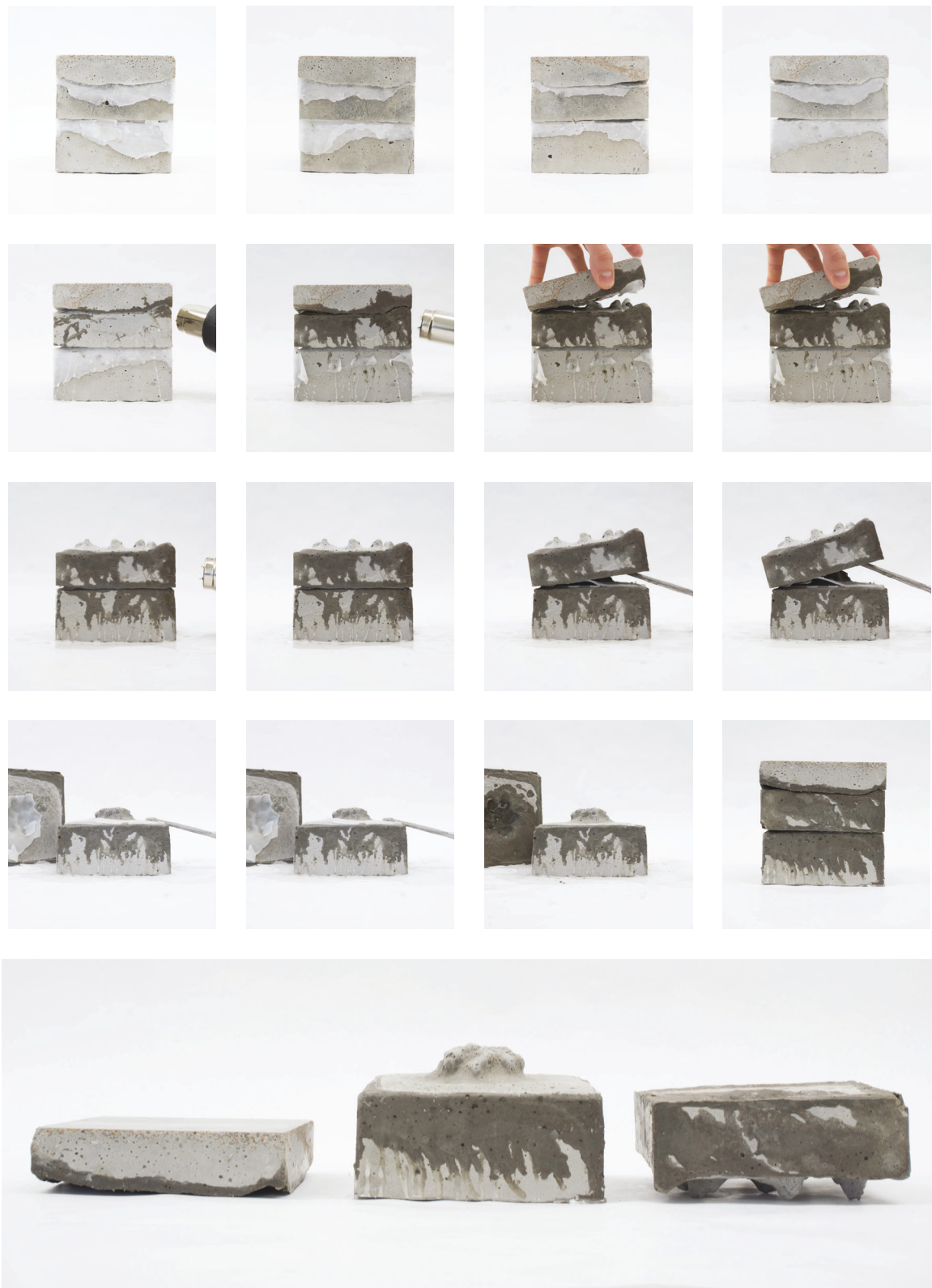
Investigation 5.2 - Sequence of melting and disassembly
