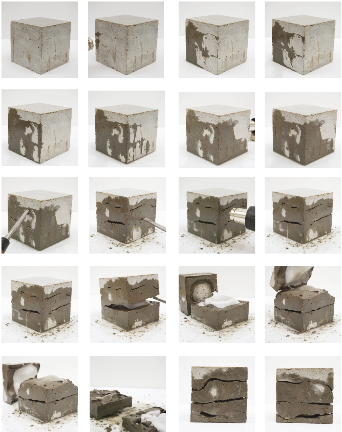
Investigation 5.1 - Sequence of melting and disassembly
