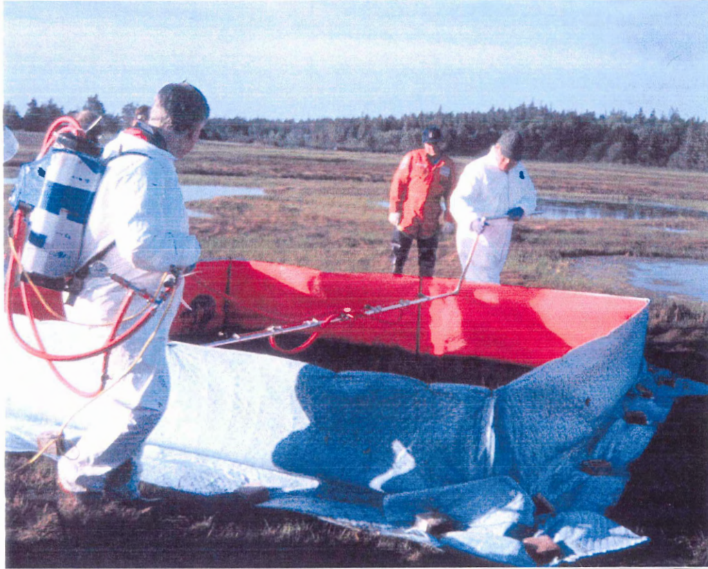
Fig. 3.3 Oil-spray boom system with backpack sprayer
