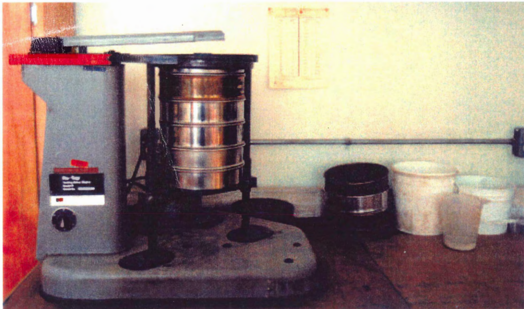
Figure 3.3: Ro-Tap Sieve Shaker; samples are placed into the upper sieve and are shaken through a series of downwards fining sieve sizes to produce a grain size distribution for the sample.
