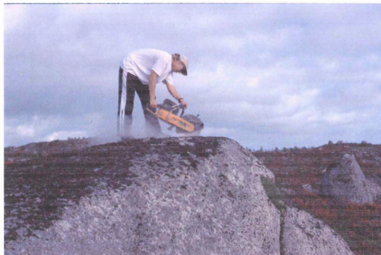
Figure 19 Example of a typical wind swept ridge, NS-PEGGY-02-009, also showing the use of a cutoff saw to help collect samples.
