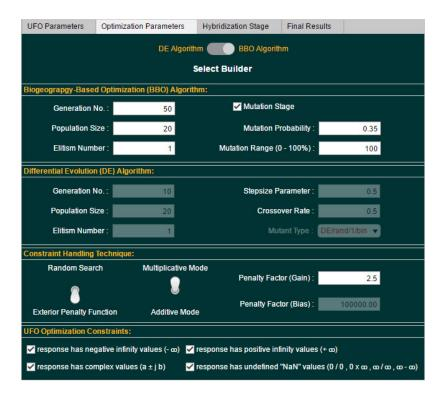
Figure 10.12: The Second GUI Tab. It is Used to Adjust the Building Stage and Its Associated Design Constraints
