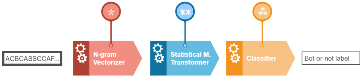
Figure 3.2: Experimental setup for bot detection task. *N-gram sizes with length setting 1–4; **5 statistical measures; ***5 different classifiers.
