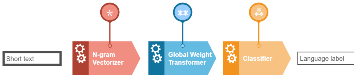
Figure 2.14: Experimental setup for language feature weighting task. *N-gram sizes with length setting 1–7, depending on a dataset; **15 weighting schemes; ***3 different classifiers: Multinomial Naïve Bayes, Logistic Regression and Linear SVM.
