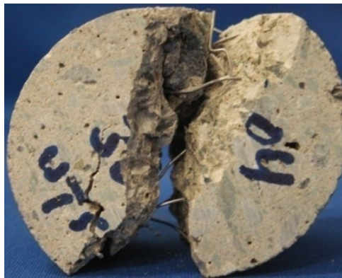
Figure 5-8 Shotcrete specimen after Brazilian test (after Saw et al., 2009)
