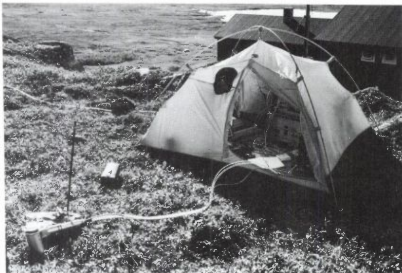
Figure 1. CO 2 /H 2 O porometer head and igloo tent with the control device north of the building of "Arktisk Station".
