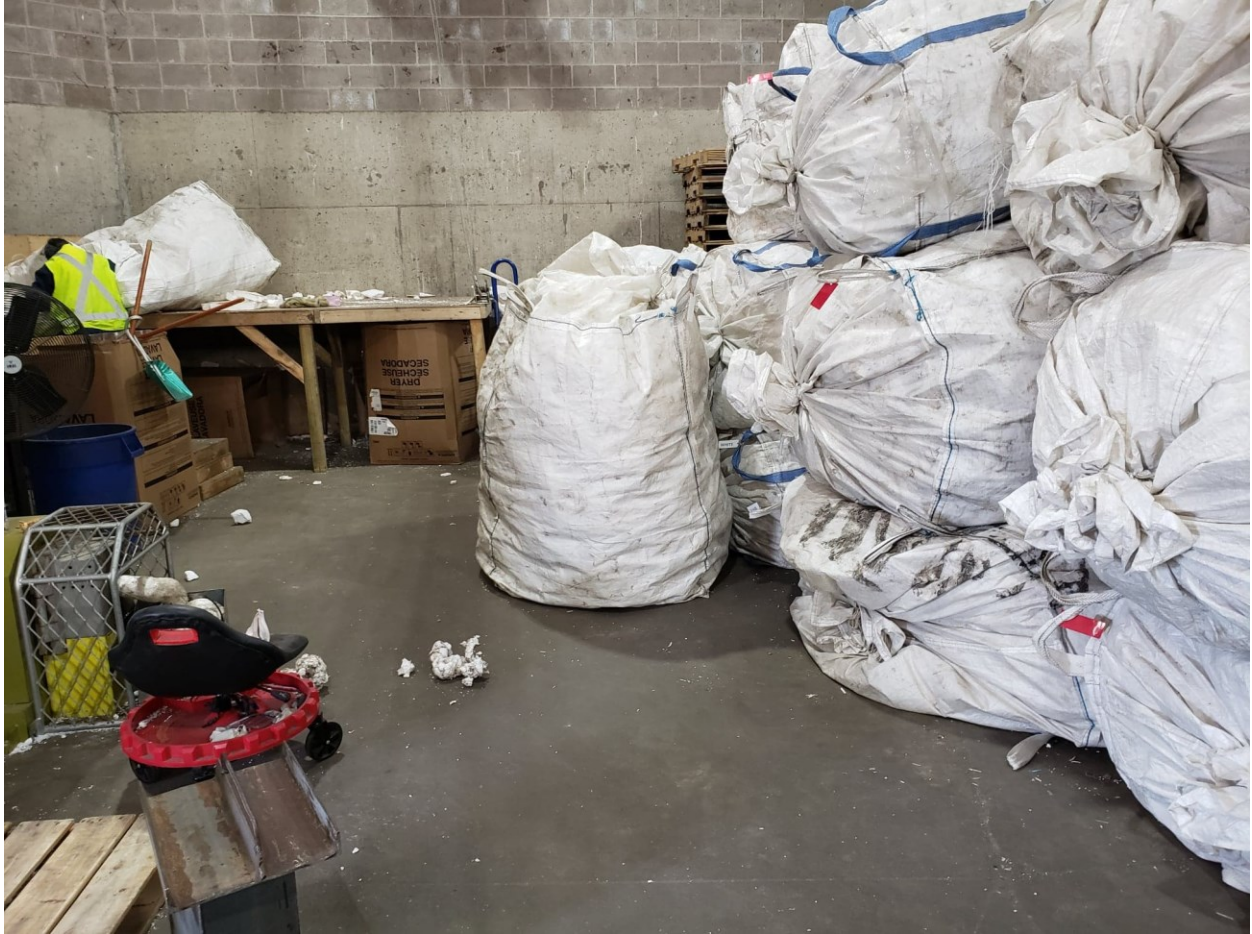
Figure D. 9 Polystyrene collected in totes prior to being densified
