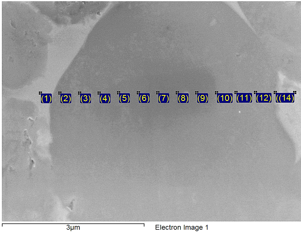
Figure 8.5 Representative SEM of TiC 17-4 PH sintered sample with 30 vol.%. Observe the core-rim structure. Table 8.2 has the spectrum the corresponds to this figure.
