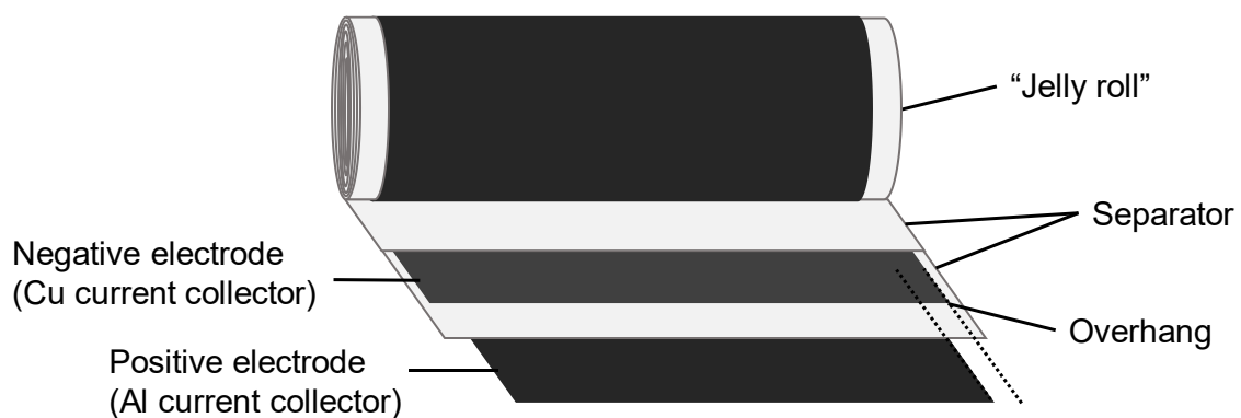
Figure 1.1: A schematic of lithium-ion cell components.
