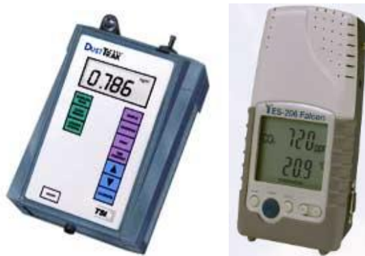
Figure 1. From left to right: DustTrac PM monitor and the YES-206 Falcon CO 2 monitor.
