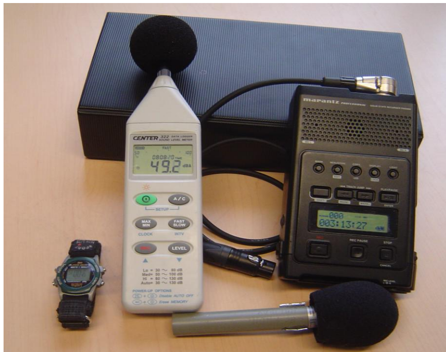
Figure 2. Center 322 SLM (white) and Marantz 660 recorder (black) with microphone, wrist watch for scale.
