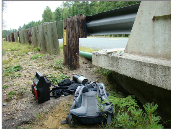
Figure 1. Unobtrusive speed observation location on the J-Line Road bridge and placement of the speed radar gun at the roads edge (between the concrete and wood post).
