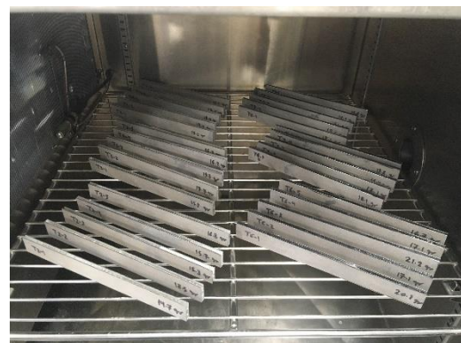
Figure 1. (a) Typical heating/cooling cycle, and (b) specimens in the environmental chamber.
