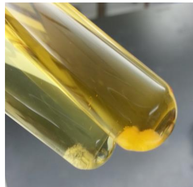
Figure 8: P samples extracted with the Golterman (1996) method as seen after preparation for measurement of P with spectrophotometer. Samples turned a brown/yellow color and a white precipitate formed.
