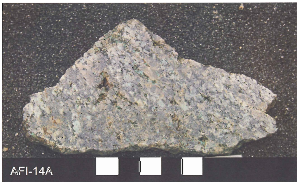
Figure 5.2: Hand specimen of sample AFI-14A. Copper oxide is visible in the rock as well as rusty vugs (scale bar is in cm).
