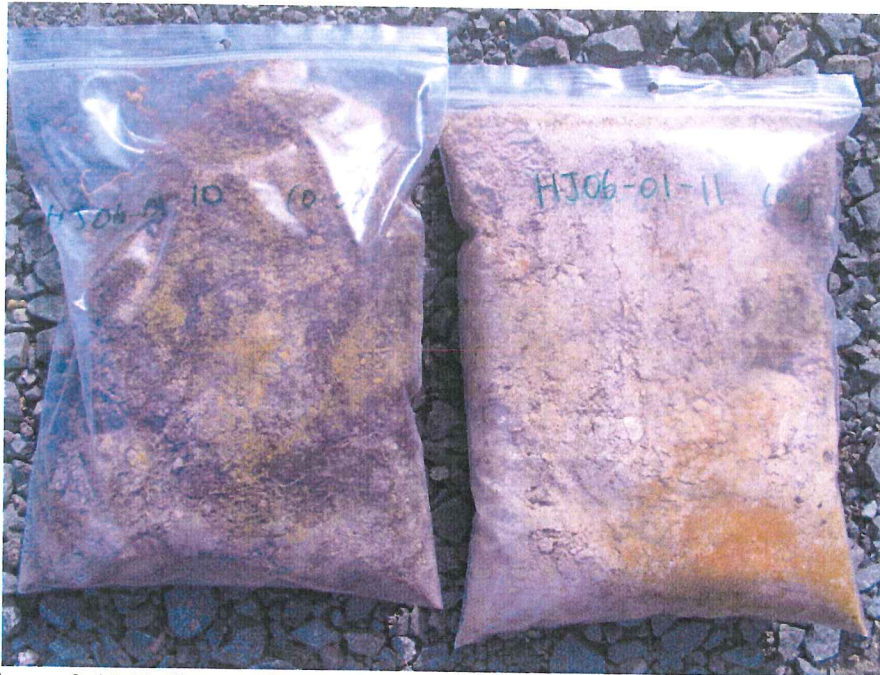
Figure 3.11 Bulk samples from the up-ice sampling location. The left sample bag contains the top 5 cm of the horizon and the right sample bag contain the top 30 cm. Notice the mixture of various soil horizons observable by the mottled colour (Photo taken by T. Goodwin, 2006).
