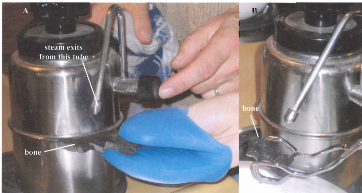
Figure 3.2: Using a cappuccino maker to remove glue. Gloves are used to handle the larger bones (A), while tongs are used for the smaller bones (B). The steam is not visible in the photos.
