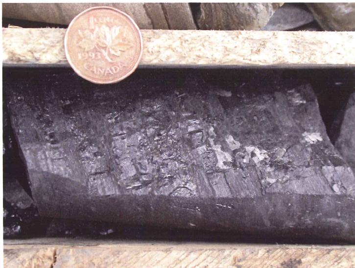
Figure 3.1 a-b. a) Coal seam (1a) cropping out south of the Debert River bridge near Cottam Settlement. Hammer is approx. 25 cm for scale. b) Close-up view of a piece of high volatile A bituminous coal (1a) from drill core DDNSD-2. Note penny for scale.
