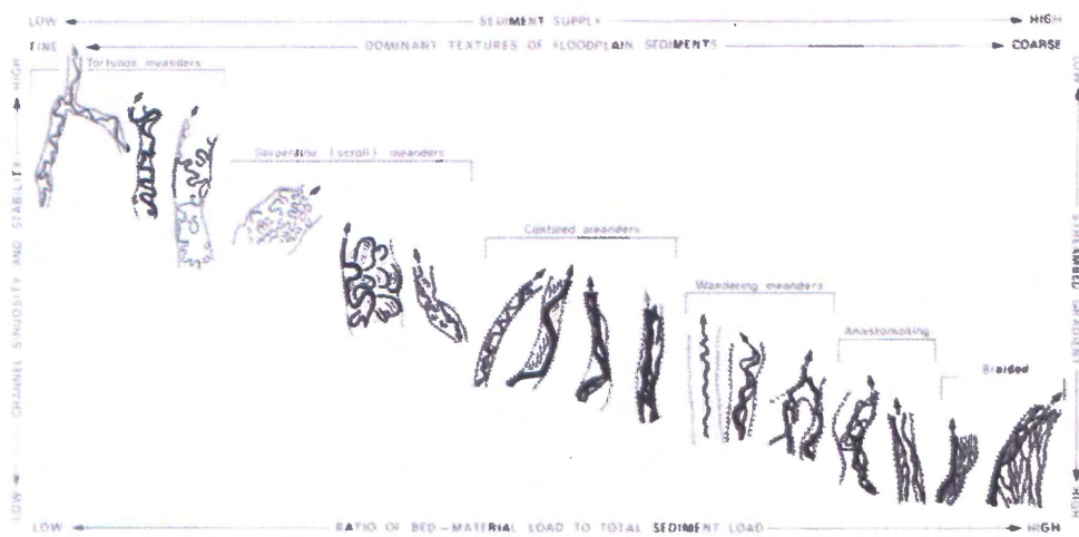
Figure 2.8 Diagram showing how channel morphology changes as aspects like sediment supply, bed load, channel stability, and stream gradient change and the resultant channel style (Taken from Selby 1985).
