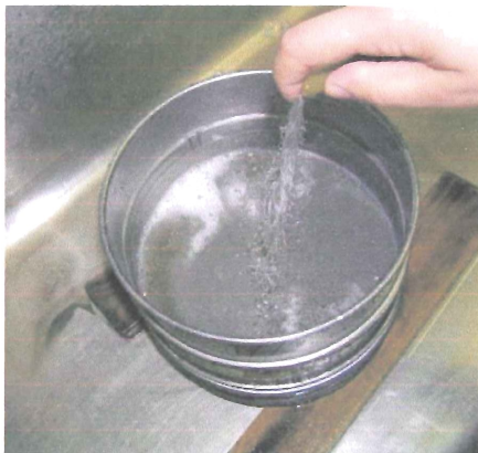
Figure 2.5A: A sample being washed with water and sieved at > 63 \mu and > 45-63 \mu .
