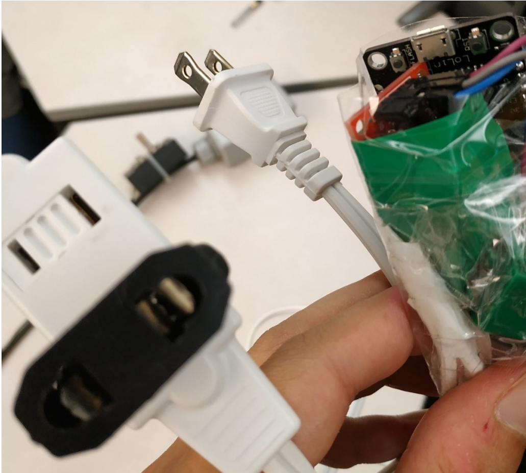
Figure 29 Device Control Module: Microcontroller, and Controlled Socket
